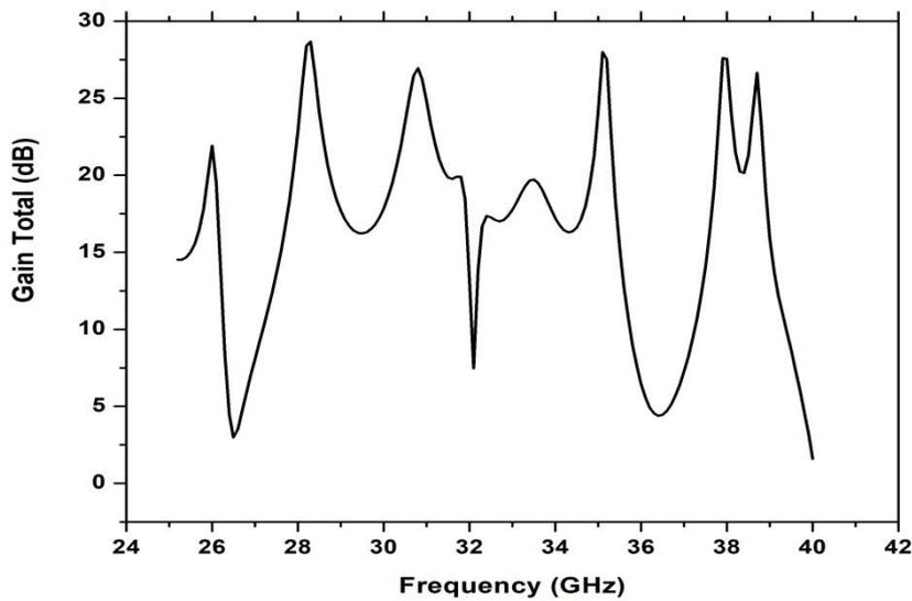
**Figure 5 Gain Curve of proposed antenna**
