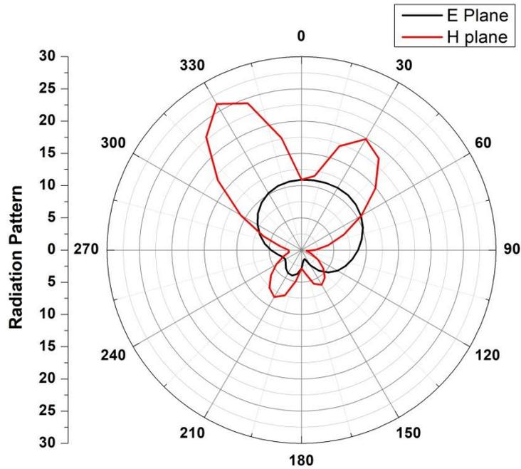
**Figure 4. E and H Plane Radiation Pattern at 26 GHz**
