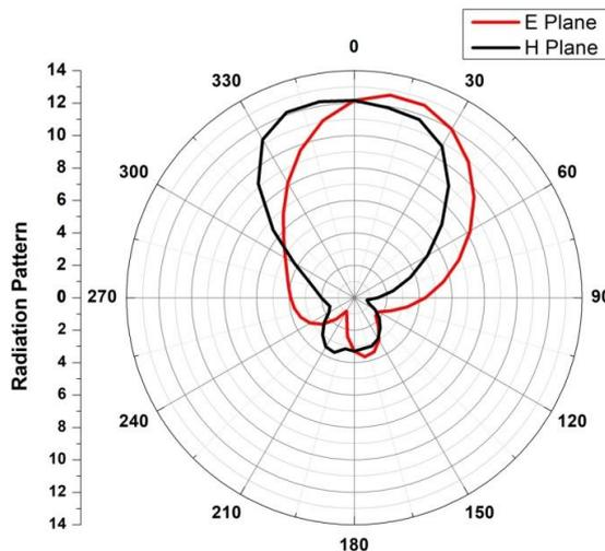
Figure 3. E and H Plane Radiation Pattern at 28 GHz
