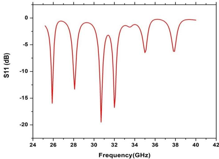
Figure 2. Return loss curve of SIW antenna
