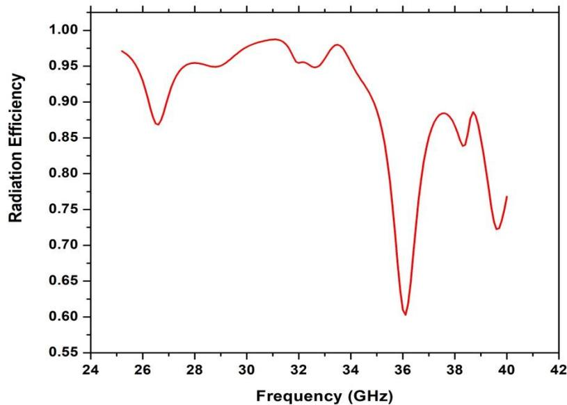
**Figure 5 Radiation Efficiency Curve of proposed antenna**
